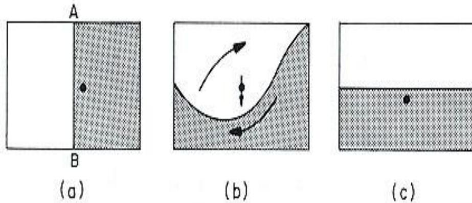
Fig. 9.1 (a) Heavier (shaded) and lighter fluids separated by a movable partition AB. The dot represents the center of gravity of the two-fluid system. (b) Fluids in motion following the removal of the partition. (c) Equilibrium configuration of the fluids after the motion has been dissipated by friction.
