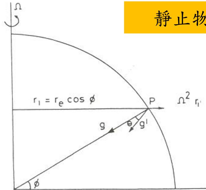
Figure 7.1. Centrifugal acceleration on a particle stationary with respect to the Earth.  $g'$  (effective gravity vector) is the resultant of the centrifugal acceleration and gravity,  $g$ .
