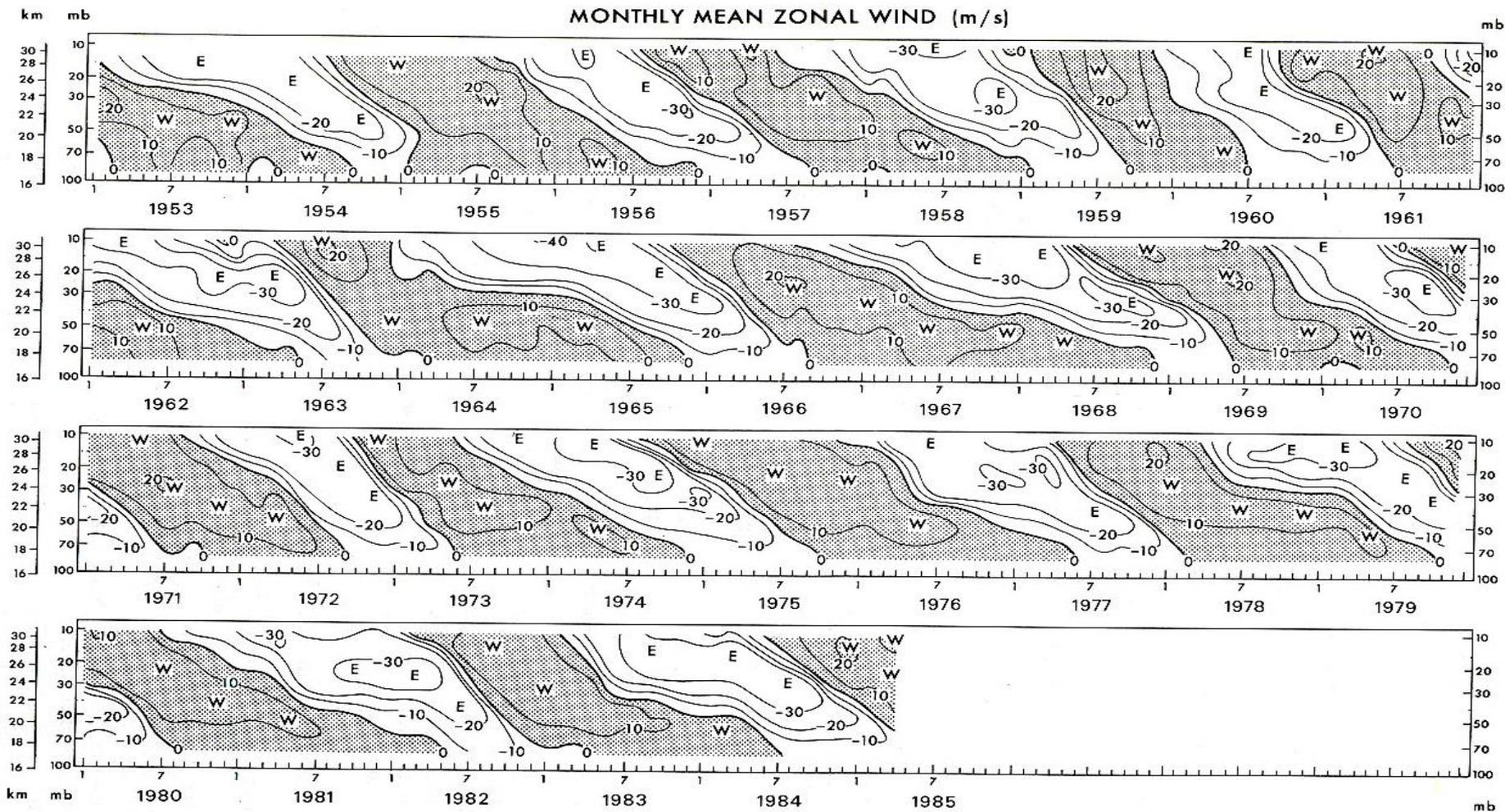
**FIGURE 16.1.** Time-height section of the monthly-mean zonal wind component near the equator in  $\text{m s}^{-1}$ , showing the QBO signal of alternating westerly and easterly winds. The section is based on data from Canton Island ( $3^{\circ}\text{S}$ ,  $172^{\circ}\text{W}$ ; 1953–1967), Gan ( $1^{\circ}\text{S}$ ,  $73^{\circ}\text{E}$ ; 1967–1975), and Singapore ( $1^{\circ}\text{N}$ ,  $104^{\circ}\text{E}$ ; 1976–1985) (after Naujokat, 1986).
